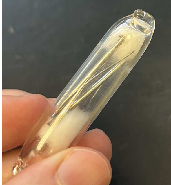
Figure 4.16: Sealed hafnium source and witness samples before irradiation at McMaster in March 2025.
