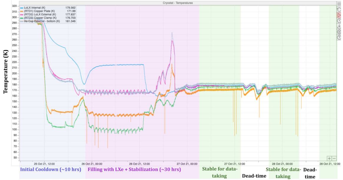
Figure 2.11: MIDAS Slow control temperature readout of the LoLX phase-1 October 2021 LXe run. Overlaid highlights show pre-run cooldown, LXe filling and data-taking periods. Extensive instability is clear during the filling cycle, with additional spikes during LN 2 re-fill cycles, shown as dead-time windows.
