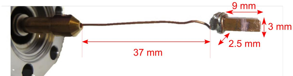
**Figure 3.6:** Image of the rectangular Cu sample attached to the CF 1.33" feedthrough flange. Dimensions of the Cu holder and the target itself are shown in red.
