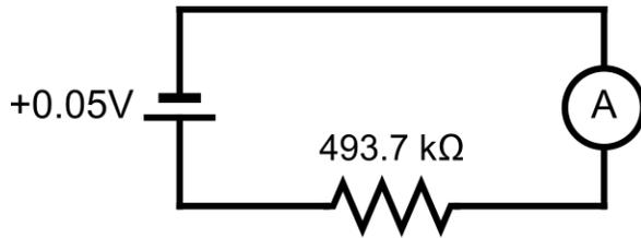
**Figure 4.4:** Circuit to study current data acquisition. 0.05 V were applied from an external power supply to a  $493.7 \pm 0.1 \text{ k}\Omega$  resistor, leading to a current measurement of  $\sim 100 \text{ nA}$ .
