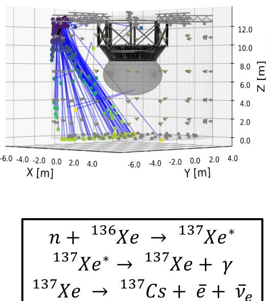
nEXO's Muon Veto System For nEXO, a 12.3-meter diameter, 12.8-meter high water tank containing 1.5 kilotonnes of ultra-pure water is designed to serve as the experiment's outer detector. The tank is equipped with 125 photomultiplier tubes (PMTs) to detect the Cherenkov light.
