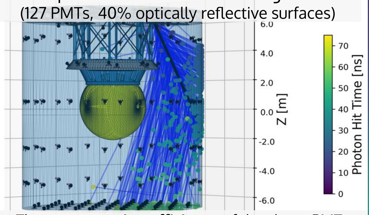
The muon tagging efficiency of the above PMT configuration is **84.4** ± **0.7** %. A uniform PMT distribution yields: 76.9 ± 0.8 %.
